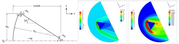
Fig. 3 (a) (left) Sketch of Apollo reentry capsule; (b) (middle) Simulated density contour with surface pressure; (c) (right) Simulated temperature contour with surface heat flux.
