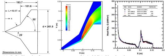
Fig. 2. (a) (left) Sketch of 25-55° double cone; (b) (middle) Simulated temperature contour; (c) (right) Comparison of present simulation with previous published data.
